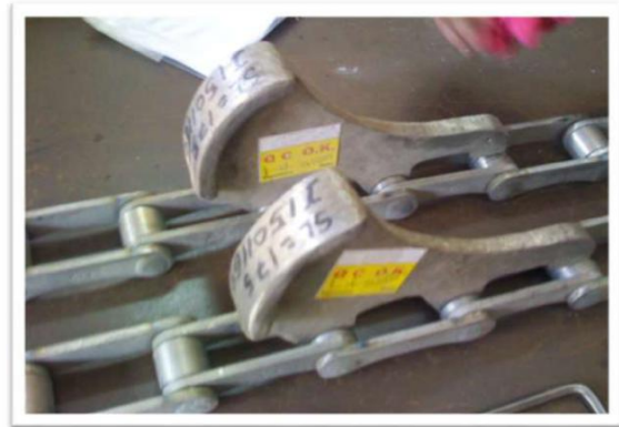
High Heat Resistant Transfer Conveyor Chains for Hot & Cold Zone of Carburizing, Carbo Nitriding, Hardening & Sealed Quench Furnaces.
