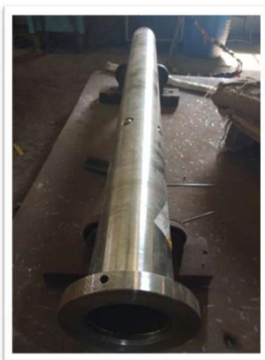
Radiant Tubes for Gas Fired Furnaces to Transfer Heat Load.
