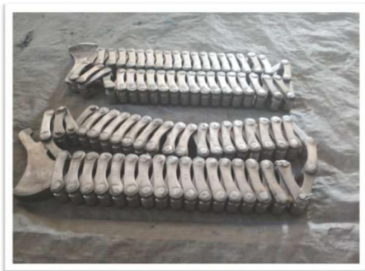
High Heat Resistant Transfer Conveyor Chains for Hot & Cold Zone of Carburizing, Carbo Nitriding, Hardening & Sealed Quench Furnaces.
