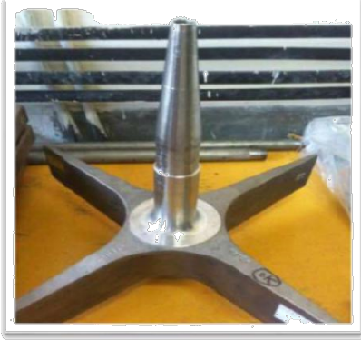
Single Piece Dynamically Balanced Fan Impeller used in Sealed Quench Furnaces which is mounted on Bung Roof of the Furnace.
