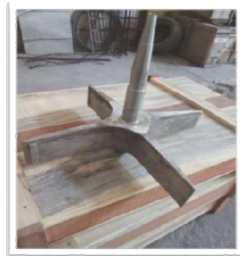
Single Piece Dynamically Balanced Fan Impeller used in Sealed Quench Furnaces which is mounted on Bung Roof of the Furnace.
